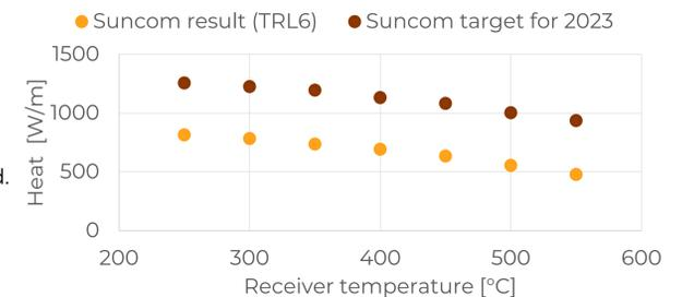
Figure 4: Current net heat output versus target for 2023
